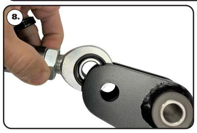
**8.** Align the mounting holes with the through hole of the rod end. Install a 5/8" flat washer on a  $5/8"-18 \times 2 1/2"$  bolt. Insert the bolt/ washer though the aligned holes. Assemble both bars & pivots.
