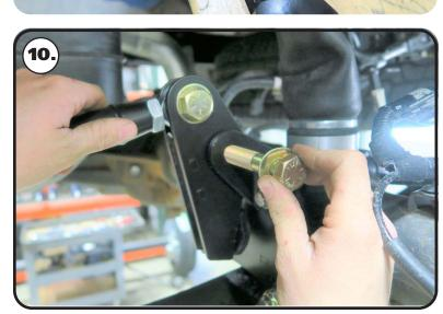
**10.** Insert the pivot/bar into the axle mount. The pivot needs to be installed with the bar at the top and the bumpstop to the axle mount. Install a 5/8" flat washer on a 5/8"-18 x 3 3/4" bolt. With the mounting holes aligned with the pivot inner sleeve, insert the bolt/washer. Install a 5/8" flat washer & 5/8"-18 nylok nut on the bolt. Torque to 115 ft-lbs.
