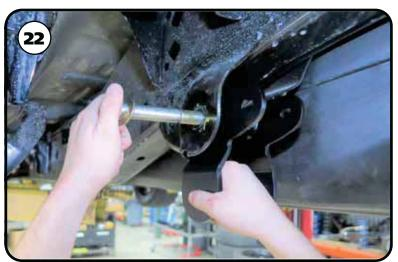
**22.** Install a M18 flat washer on a M18-2.5 x 130mm bolt. Insert the bolt into the OEM leaf spring hole. Install a M18 flat washer & M18-2.5 nylok nut on the threads of the bolt. Do not tighten at this time.
