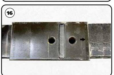
**16.** The new shims have the holes offset to the front of the truck. The arrow on the shim should point to the front of the truck. Replace the bottom and middle shims that are indicated in **Step 14**.
