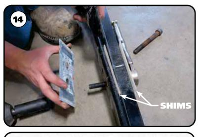
14. The top shim will also be discarded. The CENTER & BOTTOM shims will need to replaced with the offset ones supplied in the kit. Steps
