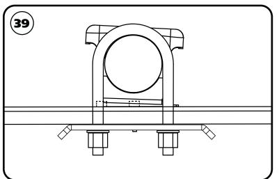
**37.** Slip the U-Bolts over the axle tube with the threads pointing down.
