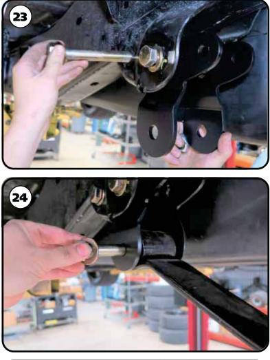
**23.** Make sure the holes in the front tab line up with the front hole of the OEM leaf spring mount. Install a 3/4" flat washer on a  $3/4"-16 \times 5"$  bolt. Insert the bolt/washer through the front hole of the leaf spring mount. Install a 3/4" flat washer & 3/4"-16 thin nylok nut on the threads of the bolt. Torque the hardware to 75 ftlbs.
