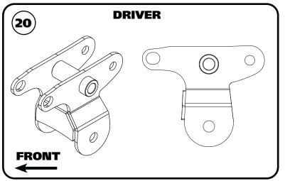
**20.** The kit includes brackets to relocate the front of the leaf spring. The brackets have a "D" or "P" stamped into the side of the bracket. The Driver side is shown in **Image 20**. The bracket is mounted in the truck with the cross tube to the top and the long tabs to the front of the truck.
