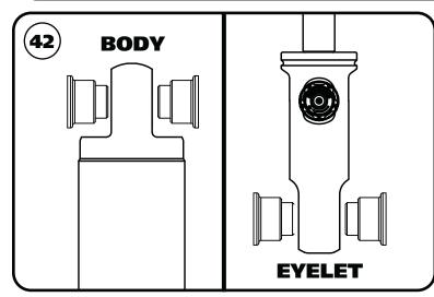
**42.** Insert the SMALL end of the bearing spacers into the shock bearings.
