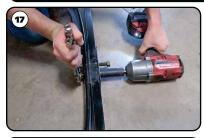
**17.** Put the new offset shims in position with the arrows to the front of the truck. Align the holes in the springs and shims and reinstall the locating pins from the TOP side. Reinstall the nuts on the BOTTOM side and tighten. Torque the nuts to 35 ftlbs Repeat on the second spring.
