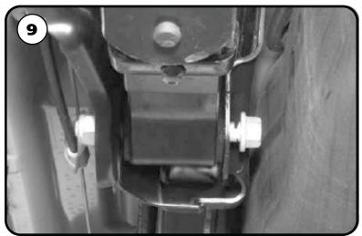
**9.** The front of the leaf springs will need to be disconnected to install the front bracket and to move the springs under the axle. Due to the location of the fuel tank and exhaust, cutting the bolt head off is the easiest way to remove it. Loosen the nut enough the expose the shank of the bolt. Push the bolt in toward the fuel tank/exhaust. Cut off the head of the bolt, being careful to not damage the fuel tank, exhaust, or frame.
