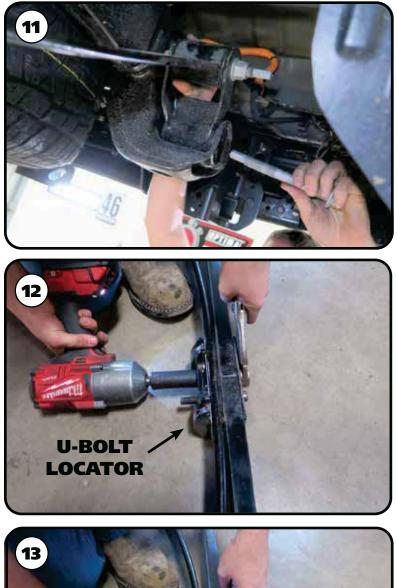
**11.** The rear of the leaf springs will need to be disconnected to move the springs under the axle and to also replace the shackle. Support the rear of the leaf spring and remove the bottom leaf spring shackle bolt. Remove the rear shackle form the leaf spring.
