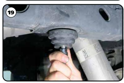
**19.** Install a M10 flat washer on a M10-1.5 x 30 mm socket head cap screw. Insert the washer/ bolt in the center hole of the bumpstop. Use a hex key (allen) wrench to attach the bumpstop in the OEM location. Repeat on the other side and torque to 35 in-lbs.
