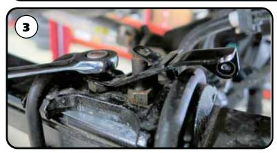
**3. 2021 & NEWER ONLY!** Disconnect the headlight sensor linkage from the Drivers side leaf spring mount. Remove the linkage bracket from the axle. There isn't a sensor on the Passenger side of the truck.
