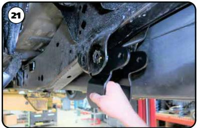
**21.** Insert the leaf spring hanger bracket into the OEM leaf spring mount. The long tabs will point to the front of the truck and insert into the OEM mount. Position the bracket so that the tube lines up with the OEM leaf spring mounting hole.
