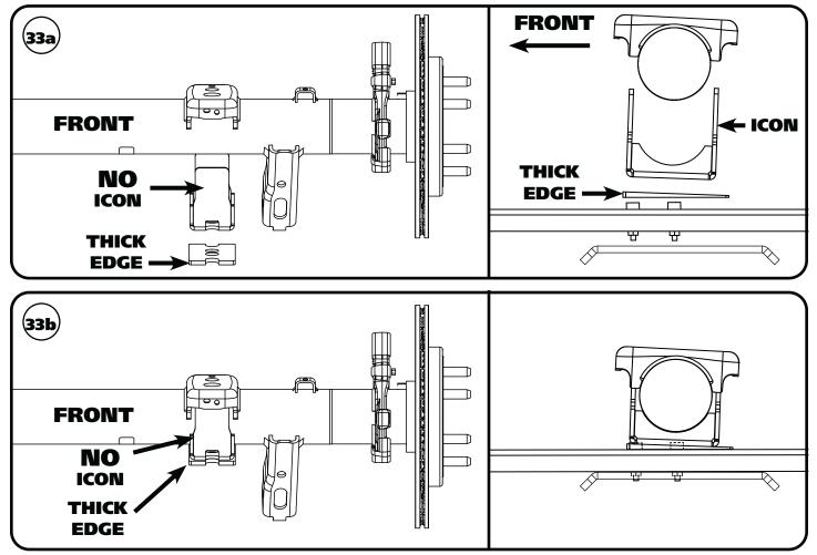
**34.** Raise the axle high enough to get the wedge shim & flip bracket positioned on the leaf spring.
