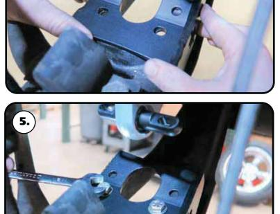
**5.** Install a 5/16" flat washer on each of (2) 5/16"-18 x 1" bolts. Insert the bolt/washer in the aligned holes of the lower mount and control arm. Install a 5/16" flat washer & 5/16" nylok nut on each of the bolts. Torque to 25 ft-lbs.
