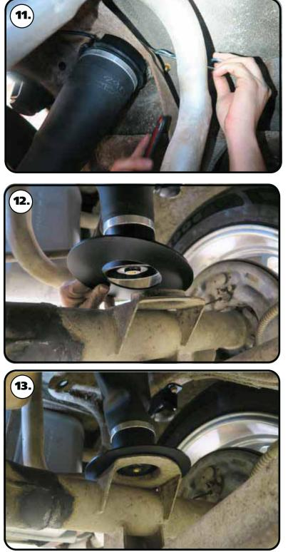
**11.** Insert the pin of the upper air spring mount through the hole drilled in the frame and the upper spacer. While holding it in place insert the long cotter pin in the hole of the pin. This will hold the air spring in place.
