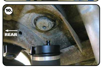
**10.** The pin of the upper air spring will get inserted into the hole drilled in previous steps. The upper mount is positioned in the car with the air fitting to the rear of the car. The pin will go through the center of the spacers installed in **Step 7**.
