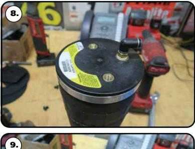
**8.** Put thread sealant on air fittings and thread them into the top of each air spring and tighten.
