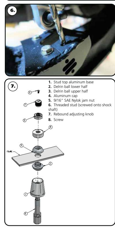
**6.** Use a 5/16" drill bit to drill the (2) inner holes using the lower mount as a guide.
