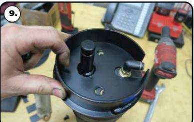
**9.** Align the upper air spring mount with the mounting holes in the top of the air spring. The upper mount is notched out to clear the air fitting. Align the notch with the air fitting and the 2 mounting holes with the mounting holes of the air spring. Install a 3/8" flat washer on each of (2) 3/8"-16 x 1/2" hex bolts. Thread the bolt/washer in the top of the air spring. Torque to 23 ft-lbs.
