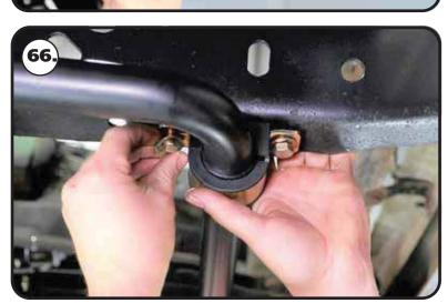
**66.** Install a 3/8" flat washer on each of (4) 3/8"-16 x 1 1/4" hex bolts. Hold the sway bar in place and insert a bolt in the mounting hole of the mounting strap. Install a 3/8" flat washer & 3/8"-16 nylok nut on the threads of the bolt. Repeat this on remaining mounting holes. Do NOT tighten the mounting bolts at this time. They need to left loose until the sway bar linkage has been attached to the lower control arm.
