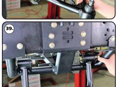
**39.** Install a 1/2" flat washer on each of (2) 1/2"-13 x 3 1/2" hex bolts. Insert the bolt/washer in the aligned holes with the threads to the rear of the truck. Install a 1/2" flat washer & 1/2"-13 nylok nut on the threads of the bolts. Re peat on the passenger side control arm. Torque the mounting bolts to 75 ft-lbs.
