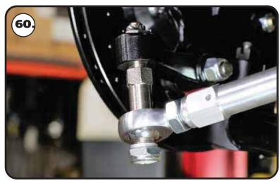
**60.** Install a 1/8" thick aluminum on the bottom side of the heim end followed by a 5/8"-18 thin nylok nut on the stud. Torque the nut to 45 ft-lbs.
