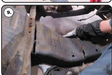
**9.** The OEM i-beam cross member will need to be cut out of the truck. It needs to be cut out even with the top of the frame rail. We also cut the cross member in the center for easier removal. We used a saw-z-all to cut the cross member out of the truck.
