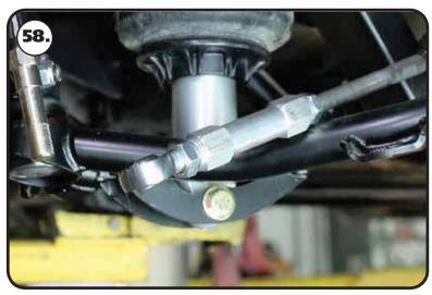
**58.** The tie rod adjusters have (2) different thread sizes, 5/8"-18 LH & 9/16"-18. The left hand threaded heim will thread into the 5/8"-18 end. The rack threads into the 9/16"-18 end. Install the 5/8"-18 LH jam nut on the heim end. Install a 9/16"-18 jam nut on the threads of the rack. Thread the heim into the adjuster and thread the adjuster onto the rack.
