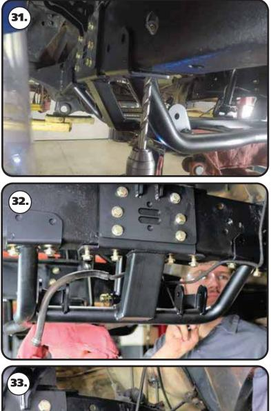
**31.** There are (8) mounting holes in the bottom mounts of each side of the cradle. All but (2) of these will need to be drilled with a 7/16" drill bit. (2) of the holes will align with factory holes.
