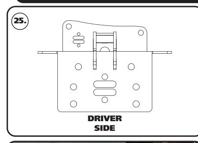
**25.** *Diagram 25* illustrates the Driver side upper control arm mount. This mount is mounted on the outside of the frame, over top the cradle The (6) holes of the upper control arm mount, align with the cradle and frame holes.
