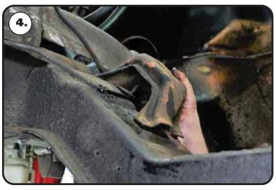
**4.** Remove the OEM engine mount stands.
