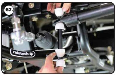
**67.** Install the end links using **Diagram 67** as a reference. Install both end links before tightening the end link hardware.
