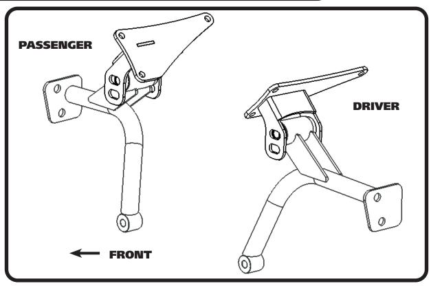
**1.** Attach the mounts to the block in the OEM location using the 10mm hardware supplied with the kit. Use the above Diagram as a reference. Torque to 35 ft-lbs
