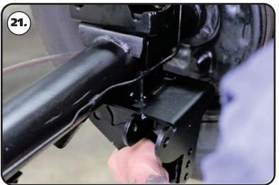
**21.** The kit includes a Driver and Passenger lower axle mount; the two are different. The Passenger mount has the panhard bar mount built into it. **Image 21** shows the Passenger mount. Hold the mount up in place against the bottom of the axle tube. The tabs will nest against the bottom of the leaf spring pad.
