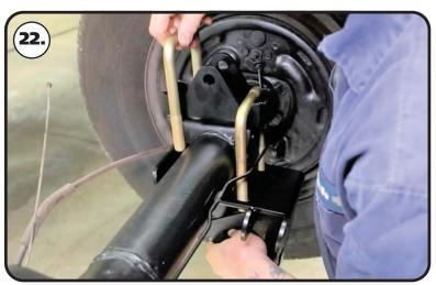
**22.** Install a supplied 5/8" u-bolt in each side of the upper bar mount. The u-bolts will nest in the slots of the upper mount. The U-bolts will run parallel to the axle tube.
