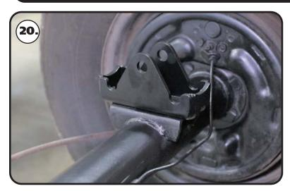
**20.** Sit the upper bar mount on the leaf spring pad of the axle. The locating pin needs to insert into the leaf spring locating hole of the leaf spring pad.
