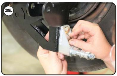
25. Insert the bolts through the axle mount and install the flat washers & nylok nuts on the threads sticking through. Repeat on both sides and torque the bolts/nuts to 75 ftlbs. Install a 5/8" flat washer onto the 5/8"-18 threads of the shock stud. Apply Red Loctite to the 5/8" threads of the stud. Thread the shock stud into the threaded hole of the lower mount. Repeat on both sides and torque the shock stud to 65-75 ftlbs.
