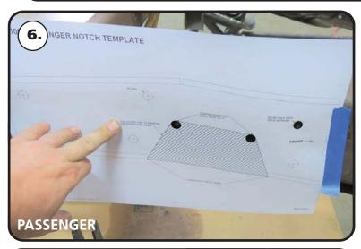
**5.** Cut the indexing holes out of the template and align them with the holes in the frame. We recommend taping the c-notch to the frame to hold it in position.
