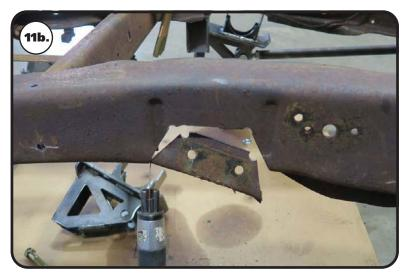
**11b.** The section of frame will fall out when cutting is complete.
