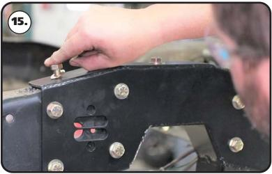
**15.** Install a 7/16" flat washer on each of (6) 7/16" x 1 1/4" bolts. This hardware gets installed in the top & bottom of the c-notch. Install a 7/16" flat washer and 7/16" nylok nut on each bolt sticking through the frame. Tighten the c-notch mounting hardware to 70 ft-lbs.
