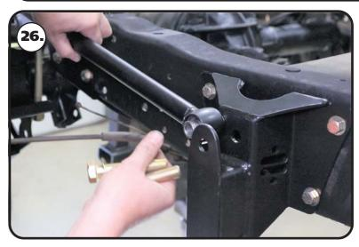
**26.** Insert (2) .625" ID x .740" long R-Joint spacers into the R-Joint of one end of each 23 7/8" center to center upper bar. The small diameter of the spacer goes into the R-joint. Insert the front of the upper bar R-Joint into the front mount. The front mount has 2 bar mounting locations. The 23 3/8" upper bar needs to be installed into the top position.
