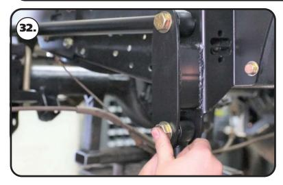
**32.** Line the through hole of the R-Joint with the of holes of the front frame mount. Install a 5/8" flat washer on to a 5/8"-18 x 3 1/2" hex bolt, insert into the lined up holes. Install a 5/8" flat washer followed by a 5/8"-18 nylok nut. Repeat on both sides and tighten the bolts/nuts enough to eliminate any gaps.
