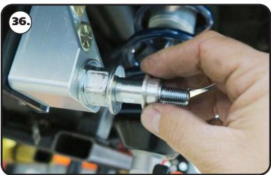
**36.** The Shock Stud requires spacers that are .400" long (90002067). Install a 5/8" ID 90002067 spacer **(Small side towards shock body)** onto the lower Shock Stud. Slide the bottom of the Shock onto the Stud. Install a second 5/8" ID 90002067 Spacer onto the Stud **(small side towards shock)**. You may need to jack the rear end up to Slide the Shock onto the Stud.
