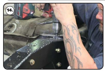
**14.** Use a 7/16" drill bit to drill the remaining holes in the top and bottom of the frame.
