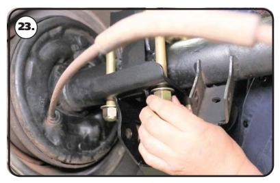
23. Hold the mount in place and install a 5/8" flat washer and 5/8"-18 nylok nut on the threads of the u-bolts sticking through the axle mount. Tighten the nuts evenly in a criss-cross fashion making sure the tabs of the axle mount are touching the leaf spring pad evenly. Torque the nuts in a criss-cross fashion to 75 ftlbs. Repeat on the other side.
