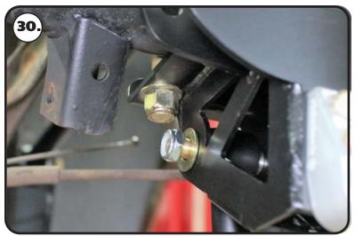
**30.** Line the through hole of the R-Joint with the of holes of the bar mount. Install a 5/8" flat washer on to a 5/8"-18 x 3 1/4" Hex bolt, insert into the lined up holes. Install a 5/8" flat washer followed by a 5/8"-18 THIN nylok nut. Repeat on both sides and tighten the bolts/nuts enough to eliminate any gaps.
