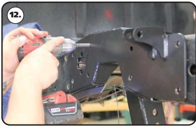
**12.** After cutting, slip the c-notch over the frame to check the fitment. The cut areas of the frame may require grinding for the c-notch to fit. The c-notch will be used as a template to drill the remaining mounting holes. Use a 7/16" Drill bit to drill the holes in the side of the frame. There are 8 holes in the side that need to be drilled.
