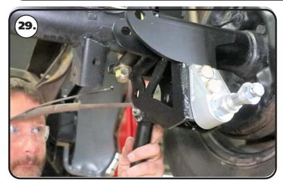
**29.** Insert (2) .625" ID x .740" long R-Joint spacers into the R-Joint of one end of each lower bar (23 5/8"). The small diameter of the spacer goes into the R-joint. Insert the rear lower bar R-Joint into the lower bar mount built into the axle mount.
