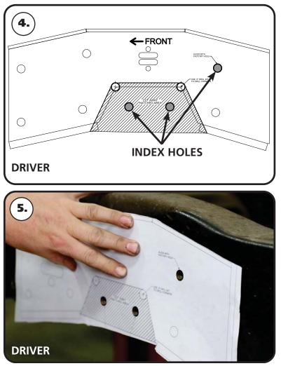
**4.** To allow maximum drop on this truck, the frame must be notched. Cutting templates are supplied with the kit to aid in cutting the frame. The template for the notch will locate off of the 3 holes that are grayed out in **Diagram "4"**. Before cutting out the frame, support the frame in front of and behind the "C" Notch area. We suggest doing one side at a time. The template has an Arrow on them that will point to the frame for wires or lines before drilling or cutting.
