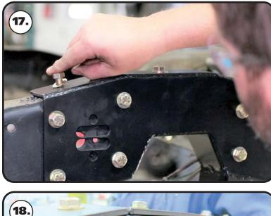
**17.** Install a 7/16" flat washer on each of (5) 7/16" x 1 1/4" bolts. This hardware gets installed in the top & bottom of the c-notch. Install a 7/16" flat washer and 7/16" nylok nut on each bolt sticking through the frame. Tighten the c-notch mounting hardware to 70 ft-lbs.
