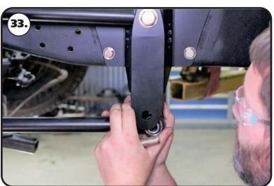
**34.** Line the through hole of the R-Joint with the of holes of the front frame mount. Install a 5/8" flat washer on to a 5/8"-18 x 3 1/2" hex bolt, insert into the lined up holes. Install a 5/8" flat washer followed by a 5/8"-18 nylok nut. Repeat on both sides and tighten the bolts/nuts enough to eliminate any gaps.
