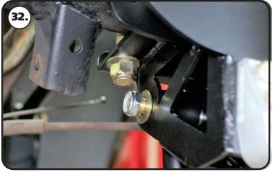
**32.** Line the through hole of the R-Joint with the of holes of the bar mount. Install a 5/8" flat washer on to a 5/8"-18 x 3 1/4" Hex bolt, insert into the lined up holes. Install a 5/8" flat washer followed by a 5/8"-18 THIN nylok nut. Repeat on both sides and tighten the bolts/nuts enough to eliminate any gaps.
