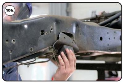
**10a & 10b.** Cut the notch with a saw-z-all, cutoff wheel, or plasma cutter. Grind all edges smooth. Cut the sides of the frame and across the bottom of the rail. The cuts on the bottom of the frame rail will be parallel with each other. The side frame cuts will blend into the drilled holes. The section of frame will fall out when cutting is complete.
