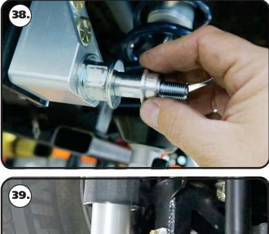
**38.** The Shock Stud requires spacers that are .400" long (90002067). Install a 5/8" ID 90002067 spacer **(Small side towards shock body)** onto the lower Shock Stud. Slide the bottom of the Shock onto the Stud. Install a second 5/8" ID 90002067 Spacer onto the Stud **(small side towards shock)**. You may need to jack the rear end up to Slide the Shock onto the Stud.
