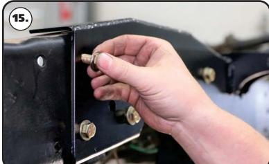
**15.** Install a 7/16" flat washer on each of (8) 7/16" x 1 1/4" bolts. This hardware gets installed in the sides of the c-notch. Install a 7/16" flat washer and 7/16" nylok nut on each bolt sticking through the frame. Tighten all of the c-notch side bolts. Tighten the hardware snuggly for the time being.
