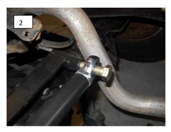
2. (fig2) Use the panhard bar as a guide to locate the panhard frame mount. At this point you should have the axle at ride height. The Panhard bar should be level at ride height. Also, you will want to verify that the rear-end is centered in the frame. The bar gets bolted to the bracket using a 5/8" x 3" bolt, flat washer, and a split lock washer.
