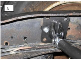
3. (fig3) This bracket can be welded or bolted to the frame using the supplied ½" hardware. Insert the R-Joint Spacers and bolt the bar to the bracket using 5/8" x 3" bolt, flat washers, & 5/8" nylok nut.
