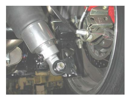
7. Bolt the lower axle bracket to the leaf spring pad using the 9/16" U-bolts and hardware supplied. Bolt the lower Shockwave mount to the axle bracket using the 1/2" x 1 1/4" bolts and Nylok nut.
