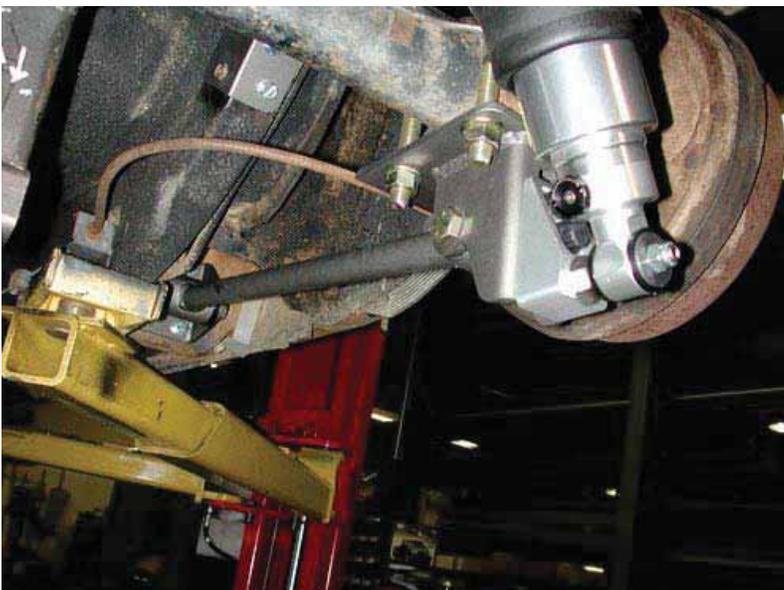
15. Apply thread sealant to a 90 degree air fitting and screw it into the top of the Shockwave. These pictures show the 9000 series Shockwave, but this kit will use the 7000 series.
