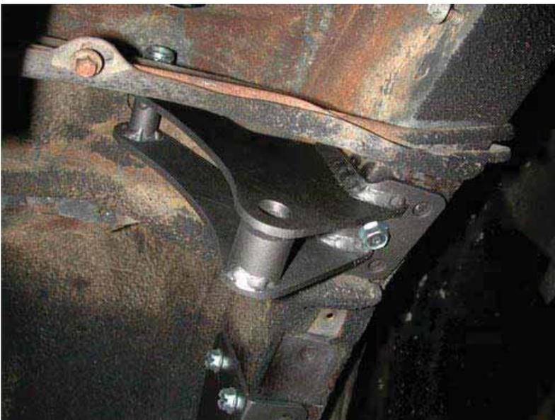
14. Attach the upper Shockwave mount to the factory upper shock mount using a 1/2" x 2 3/4" bolt, Nyloc nut, and flat washers. Swing the bracket out to the frame rail to mark and drill 5 holes in the frame with a 5/16" bit. Fasten with 3/8" x 1" thread forming bolts and flat washers.
