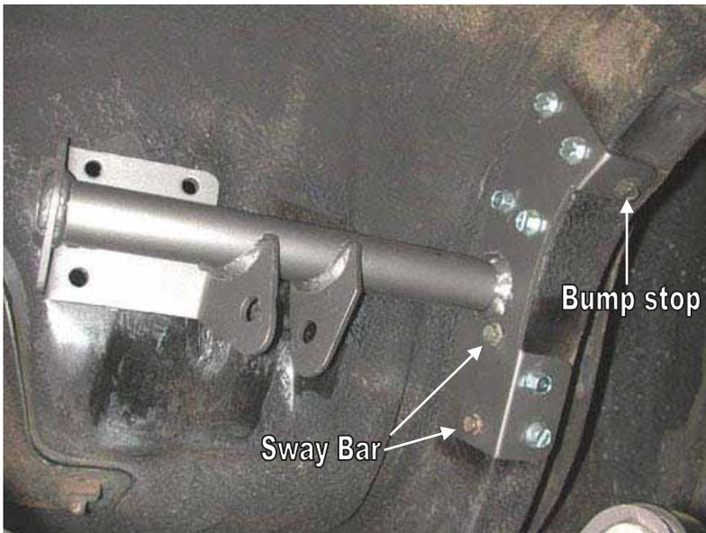
3. Place the upper bar mount up to the body. It will align off of the two sway bar mount holes and the front bump stop mount hole.
