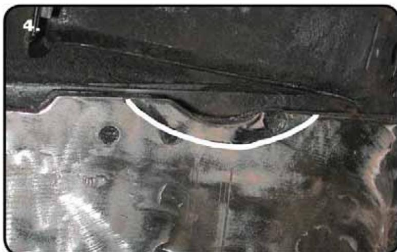
4. A portion of the frame directly behind the bump stop mount must also be trimmed for air spring clearance. This will be cut in an upside down arch down to the top of the frame rail.
