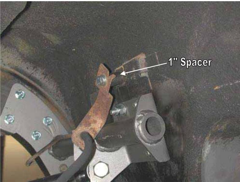
21. To remount the brake line body mount the 1" spacer is require to allow clearance with the upper bar mount. A longer 5/16" x 1 3/4" bolt, flat washer and lock washer are also supplied.
