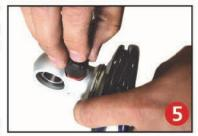
Install upper spring mount retainer clip (803-00-199) into the groove on the upper eyelet as seen in figure 5. Then, reinstall adjuster to complete assembly.
