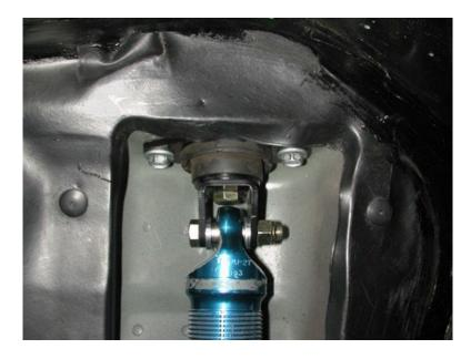
6. Bolt the eyelet to the lower control arm using the OEM Bolt & nut. The thicker aluminum spacer must be installed on each side of the bearing.
