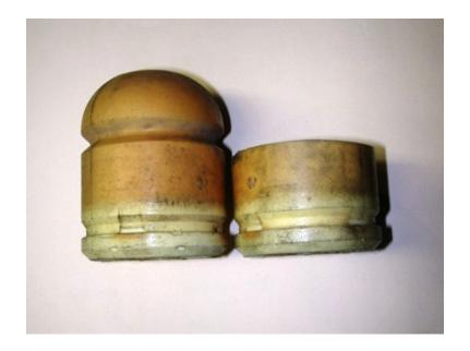
3. Remove the bump stop from the frame and cut the upper convolution off, then reinstall back onto the frame. This will allow for maximum drop.
