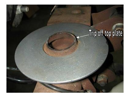
4. The top of the lower coil spring retainer must be cut off to accept the lower air spring mount. The ring will stick up past the roll plate and sticks up into the bottom of the Air spring to keep it located. A die grinder with a cut off wheel works well. Grind edges smooth.
