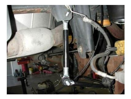
12. To retain proper sway bar geometry, shorter PosiLinks are necessary. 12mm Nylok nuts are suppled.
