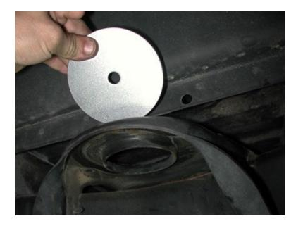
6. Place the 4" washer on top of the upper coil spring mount.
