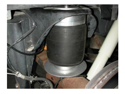
9. Place the air spring into the coil spring pocket with the 3/8" stud sticking through the 4" washer. Fasten the assembly with a 3/8" Nylok nut and flat washer.
