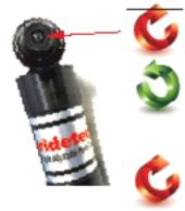
Begin with the shocks adjusted to the ZERO low speed compression position (full stiff).
