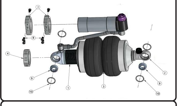
WARNING: ATTEMPTING TO REMOVE THE AIR FITTING WILL DAMAGE IT AND VOID THE WARRANTY.
