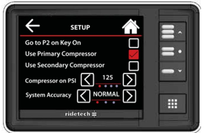
**IF YOU ARE RUNNING A 2 COMPRESSOR SYSTEM, THE 2ND COMPRESSOR WILL NEED TO BE TURNED ON IN THE SETUP MENU! YOU MAY GET ERROR #143 BEFORE YOU TURN COMPRESSOR #2 ON. IF YOU GET THIS ERROR, GO TO THE SETUP MENU AND TURN COMPRESSOR #2 ON. THE ERROR WILL CLEAR AFTER THE IGNITION IS CYCLED.**
