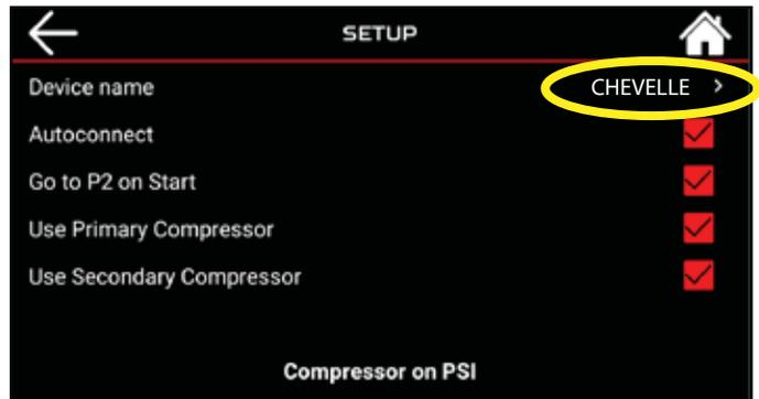
**Step 6:** The new device name will show on the Setup screen. This is also the name that will show in the Available Device screen.
