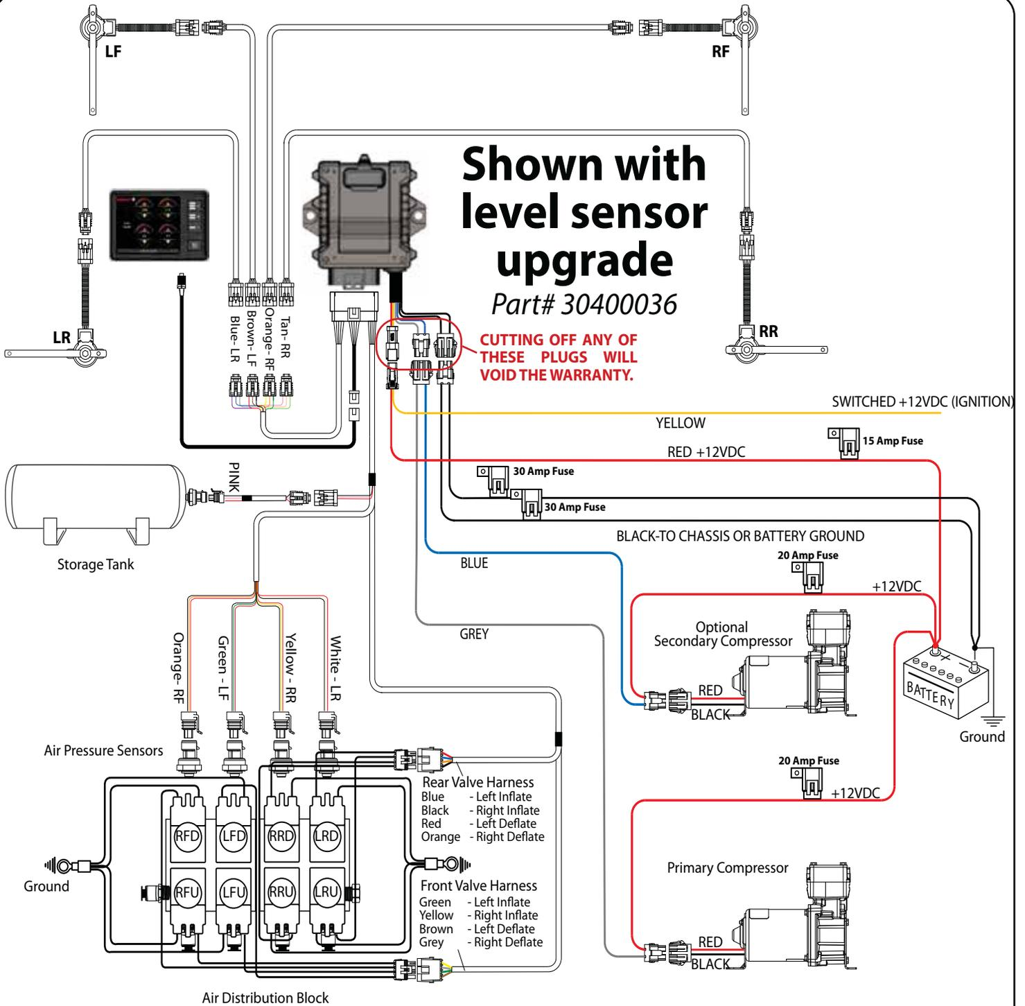
**NOTE: AIRPOD WIRING IS THE SAME, BUT THE AIRPOD HAS IT'S OWN FUSE BLOCK FOR THE ECU AND COMPRESSOR(S). THE AIRPOD STILL REQUIRES A FUSE TO BE INSTALLED AT THE BATTERY. See page 6.**
