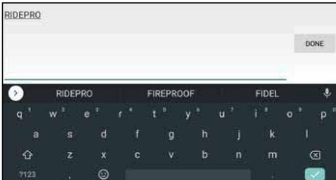
**Step 3:** A new window will pop up that has the current name of the device with a keyboard below it. Use the keyboard to delete the current name and type the new name.
