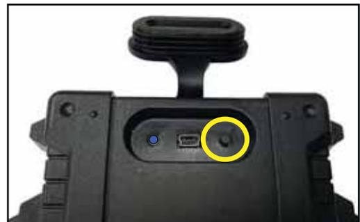
**Step 2:** Open the rubber cover on top of the ECU. Push the button that is under the rubber cover. The Blue light will start flashing.
