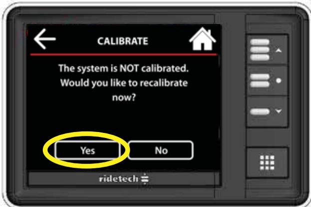
Make sure nothing is under the vehicle before performing calibration. To Calibrate the system, select "Yes".
