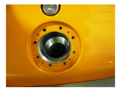
5. Remove the cap and drill the holes with a 3/16" bit.
