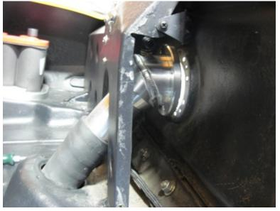
6. Factory gas tanks require a vented gas cap. This gas cap is not vented, but there is an 1/8" NPT hole tapped into the top of the filler neck that can be used to vent the tank. A hose should be used to route the fumes outside the trunk. Most aftermarket tanks are vented though; a 1/8" NPT brass plug is supplied to plug this hole.
