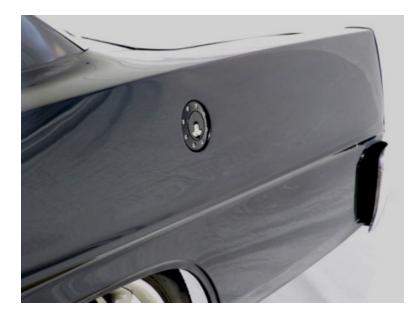
5. The factory filler neck will be reused, but the top section must be cut off to attach it to the new filler neck.
