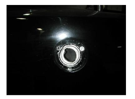
1. The factory filler neck used three screws to attach it to the tail panel. This cap will use 8 screws to sandwich the cap and filler neck to the panel.
