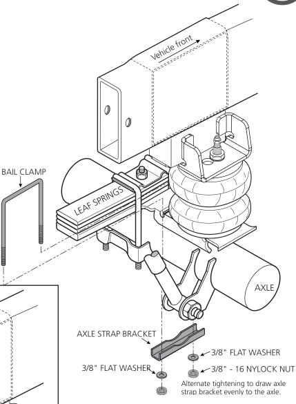
USE YOUR HAND TO CHECK FOR THE PROPER CLEARANCE AROUND THE AIR SPRING. IF YOUR HAND DOES NOT FIT BETWEEN THE AIR SPRING AND OTHER COMPONENTS, IT WILL RUB!
