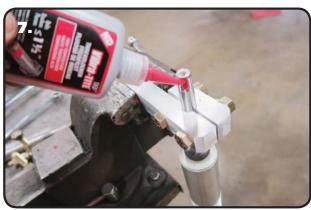
**7.** Apply Red Threadlocker to the threads of the SHOCK SHAFT. DO NOT APPLY THREADLOCKER TO THE THREADS OF THE UPPER MOUNT, it can get into the adjuster and lock it up. MAKE SURE YOU DO NOT GET THREADLOCKER ON THE END OF THE SHOCK SHAFT IN THE AREA OF THE ADJUSTER ROD.
