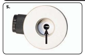
**5.** If installing an Eyelet: Check the center of the threaded hole to make sure the adjuster is threaded in far enough. You should see a small shaft going completely across the hole. You should not see any of the adjuster threads hanging out into the hole. These threads would be on the opposite side of the adjuster knob. If threads are exposed, thread the adjuster in by turning it clockwise.
