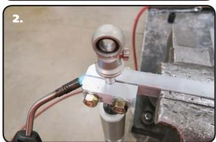
**2.** Using a Propane torch, or similar heat source, heat the Eyelet from the bottom side. Concentrate the heat in the area where the shaft goes into the eyelet. If you are removing an Adjustable Eyelet, apply heat to the side opposite of the knob.
