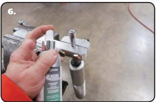
**6.** Clean the threads of the shock shaft. **Use Surface Prep Primer on both surfaces to be bonded.** Allow both surfaces to completely dry.
