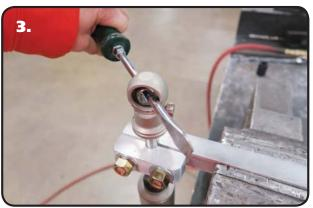
**3.** While heating the eyelet, insert a rod through the bearing in the eyelet. If you are removing a stud top, use a 3/4" wrench. Use the rod/wrench to put pressure on the eyelet as if you were trying to thread it off of the shaft. Keep putting pressure on the eyelet as you heat it until it breaks free. Thread the eyelet off the shaft. **CAUTION: THE EYELET WILL BE VERY HOT.** DO NOT REMOVE THE TOOL, IT WILL BE USED TO INSTALL THE NEW UPPER MOUNT.
