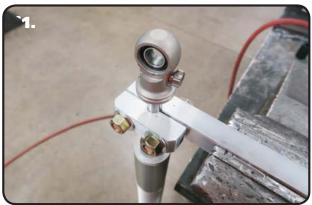
**1.** If on a CoilOver, remove the CoilSpring. If changing the Upper Mount on a ShockWave, push the AirSpring down the shock shaft to expose it. Insert the long side into a vise leaving enough room for the Shock to hang beside it. Clamp the Tool on the shock shaft below the Eyelet/Stud, shown in **Image 1**. It needs to be spaced down below the Upper Mount approximately 1". Torque the Nuts of the 2 clamp Bolts evenly to 50 ftlbs.
