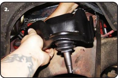
2. Insert the Ball Joint into the Control Arm from the top side of the Control Arm with the Ball Joint Pin Sticking down. Attach it to the Control Arm with the Hardware Supplied with the Ball Joint. Torque the Hardware to 14 ftlbs. Engage the Ball Joint Pin into the Spindle and install the Castle Nut Supplied. Torque the Castle Nut to 60 ftlbs and tighten to align Cotter Pin Hole. Install Cotter Pin through Hole and Bend Pins to prevent falling out.
