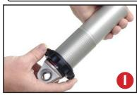
First, using the supplied lower adjuster nut (803-00-199) thread the nut onto the shock from the bottom side as seen in figure I. Remove the plastic pellet that is in the split of the adjuster nut.
