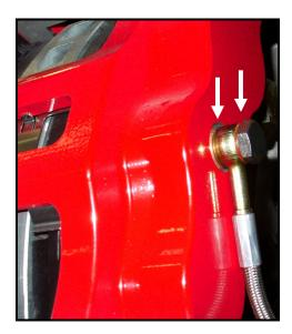
Figure 4: Installation of hose and washers
