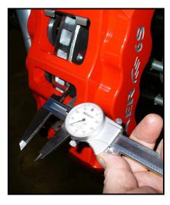
Figure 3: Measuring distance from rotor to caliper body
