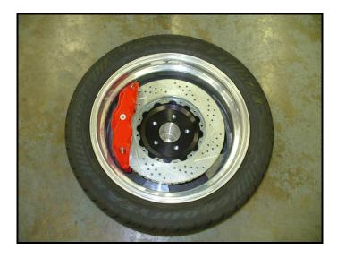
When installing new Baer rotors, be sure to follow the direction of rotation indicated on the rotor
