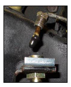
Figure 1: Hose lock location and vinyl cap installed
