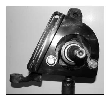
Figure 2: Rear Steer spindle shown with base bracket
